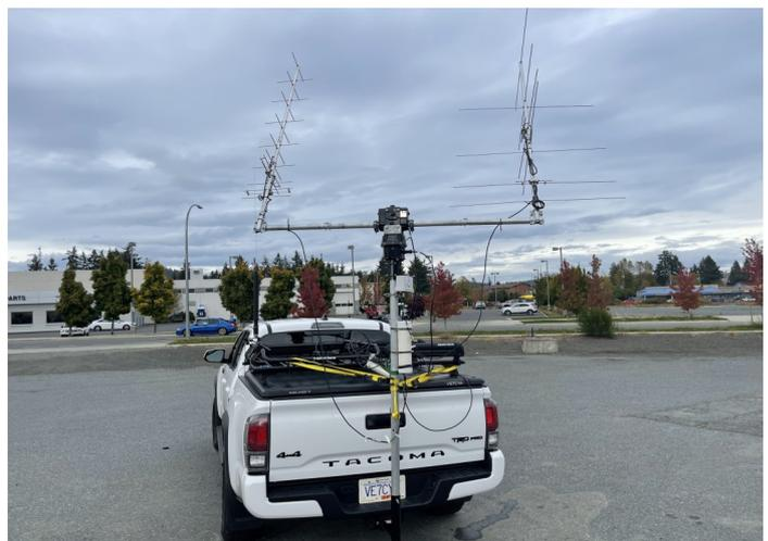
**VE7CYA’s mobile satellite station also used for roving**
