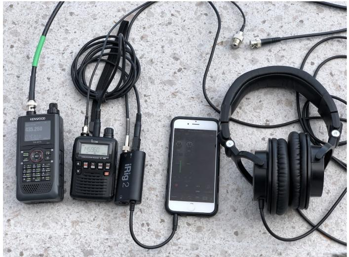
***An example of a two-radio full duplex satellite setup with an audio interface to a smartphone for recording and headphones for isolation. (OEM antennas may be used if you do not have a dual band Yagi.)***
