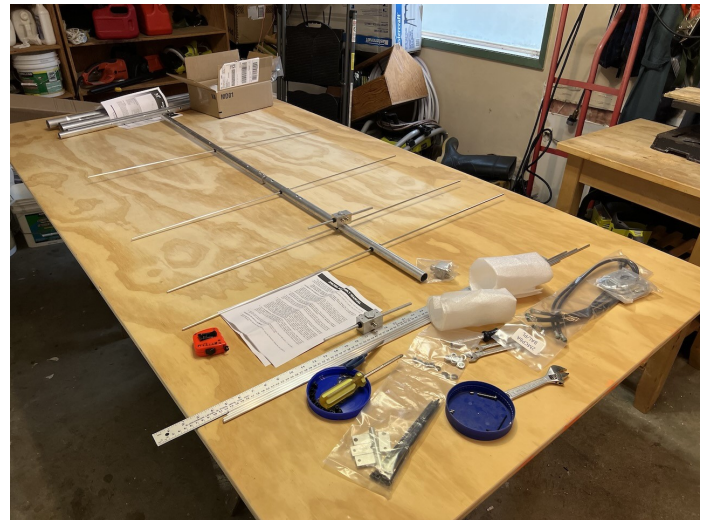
Getting started on the M2 LEO Antenna System assembly; the VHF array is half built, the remaining parts are on the right.
