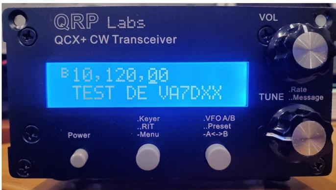
***The QRP Labs QCX+CW Transceiver can automatically display received and sent CW on the small screen***
