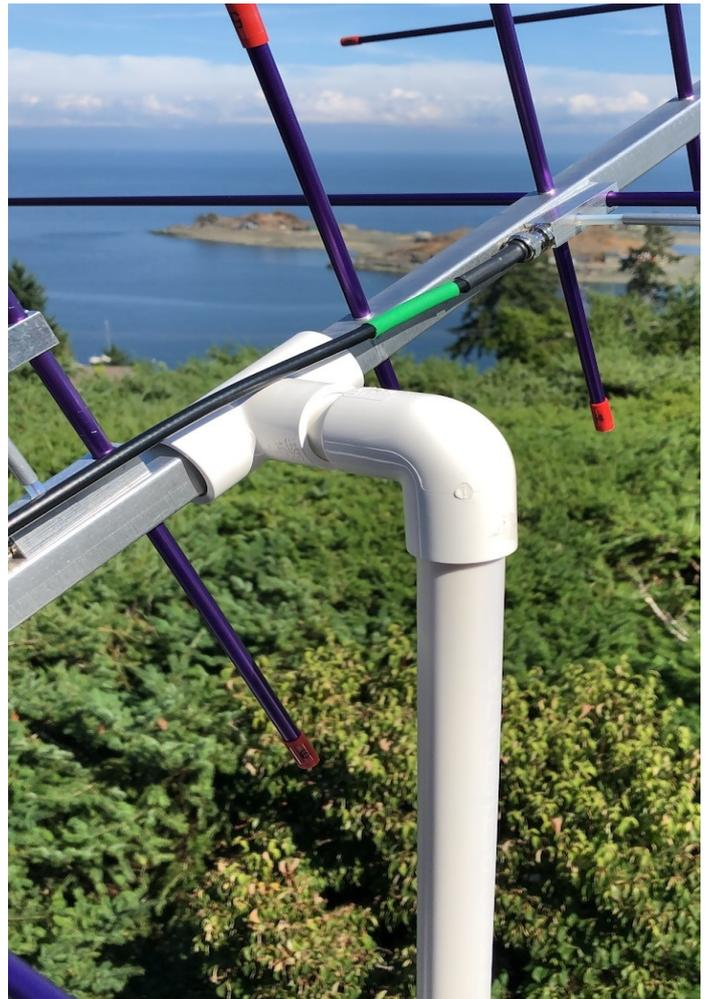
**Low-tech mount for Arrow II antenna. Built from 3/4" PVC water pipe. Joints friction-fit only to allow for repositioning. The Arrow boom is loose in the PVC tee so that it can rotate for polarization matching during the pass.**
