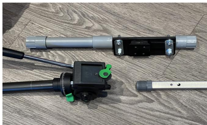
**Homemade tripod adaptor for Arrow II antenna (top). Built from 3/4" PVC conduit, ABS sheet and U-bolts with a shoe to fit the tripod head. Adapted to the Arrow's boom using a 3/4" hose barb that is stiffened with a 7/16" x 2" bolt inserted inside (not visible). The U-bolts are loose enough to allow the shaft to rotate for polarization matching during the pass**
