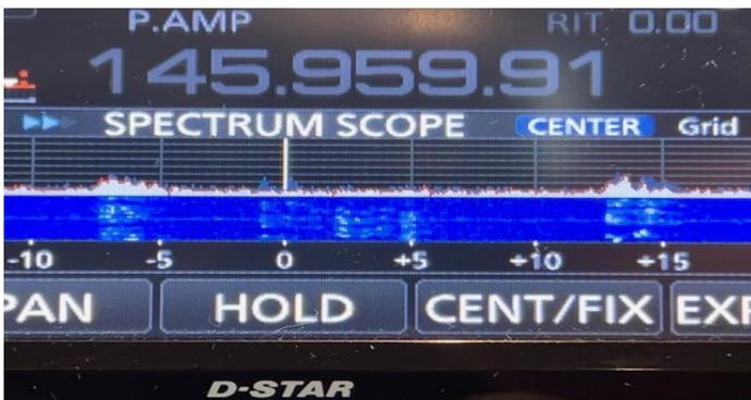
*The waterfall display of the IC-9700 during an RS-44 pass. With a bit of imagination, you can see four QSOs in progress at -7, 0, +3 and +14.*
