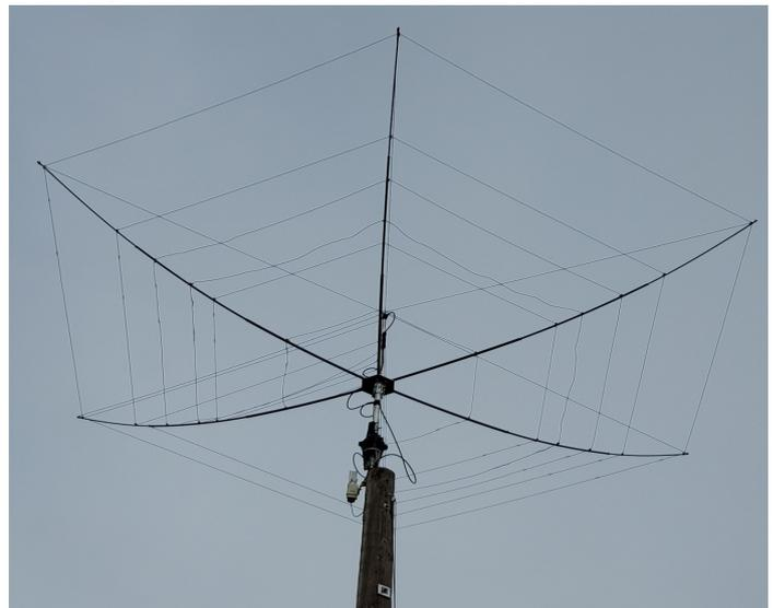
*The Hex beam mounted on the telegraph pole*
