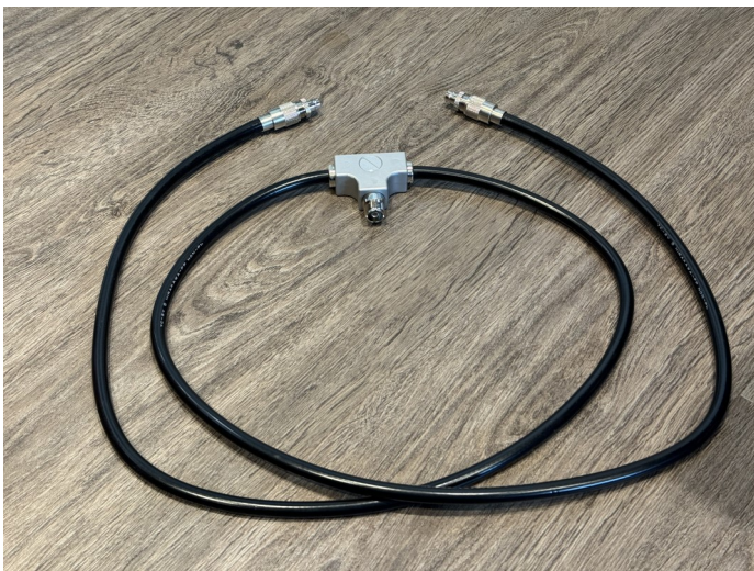
The Diamond SS770R antenna phasing harness I use to phase two Alaskan Arrow antennas. It is designed for stacking matched antennas on 2m (VHF) or 70cm (UHF) bands and can handle up to 100W
