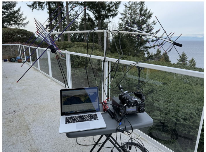
The quick-and-dirty setup of the dual Alaskan Arrow antenna system during initial test by Bruce VE7PTN
