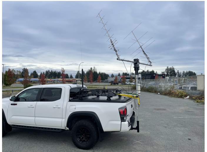
A portable version of the M2 LEO Pack antenna system in use by NARA member Ward VE7CYA
