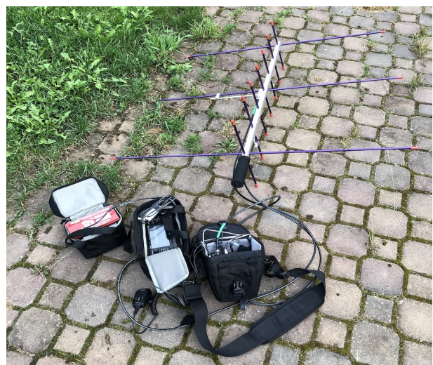
VE7PTN's motorcycle portable satellite rig consisting of an ICOM IC-705 for TX, ICOM IC-R6 for RX, an Arrow II handheld antenna, and a 10Ah LiFePO4
