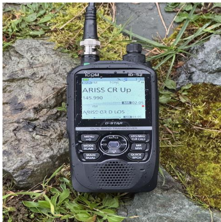
The Icom ID-52 as configured for satellite operation; the SMA antenna connector is adapted to BNC for easy attachment to the Arrow II satellite antenna.
