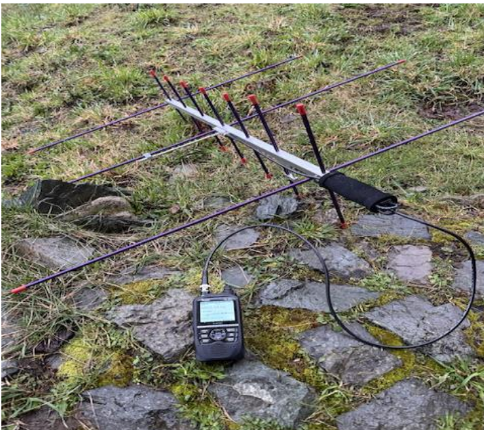
The Icom ID-52 with the full Arrow II satellite antenna. This model of antenna includes a built-in diplexer, and the boom made be broken down into two pieces for transport.
