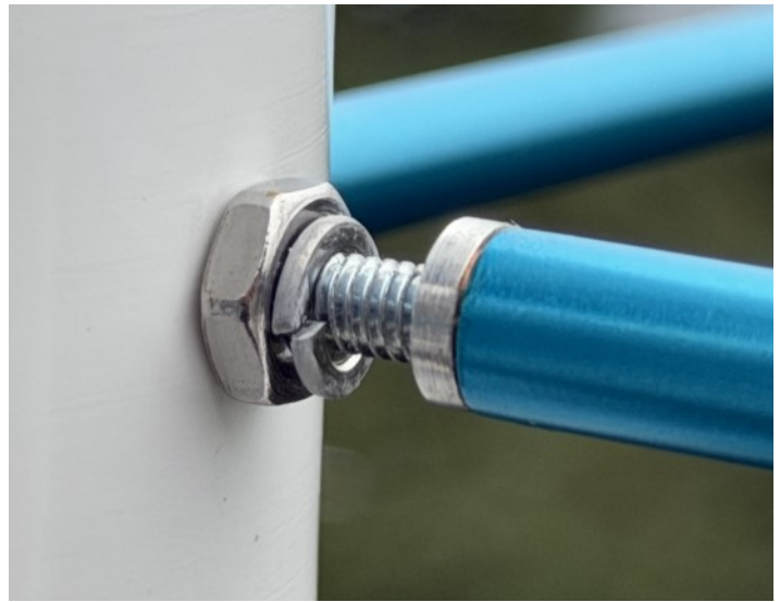
An arrow shaft element connection point on the VHF turnstile antenna built by Bruce VE7PTN. The connection is loose and shows the threaded rod and split washer used to secure the element to the antenna body.
