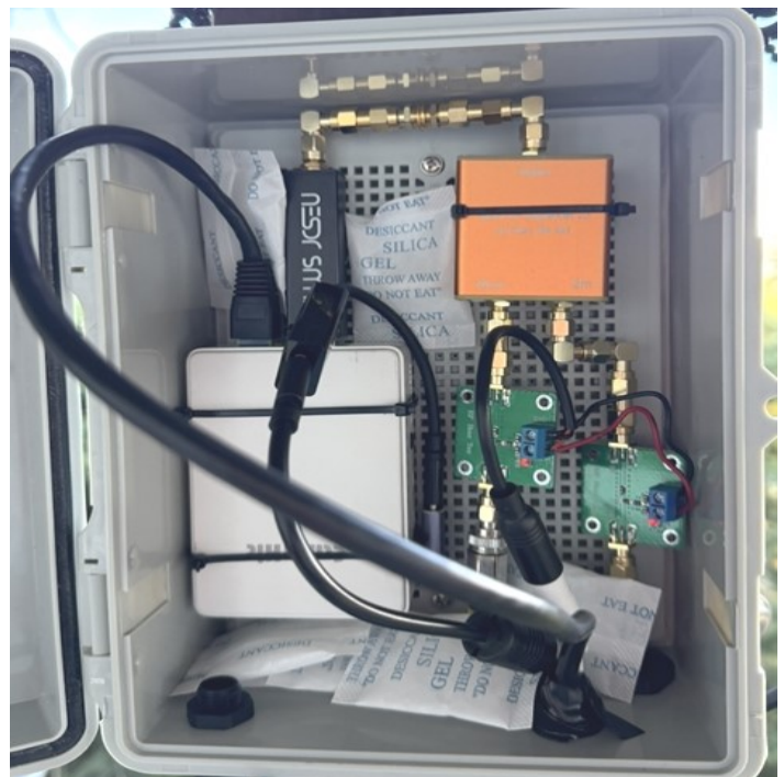
The water-resistant enclosure with Raspberry Pi, SDR, diplexer and bias tee LNA power injectors in a temporary location under the deck at Bruce VE7PTN's QTH for testing.
