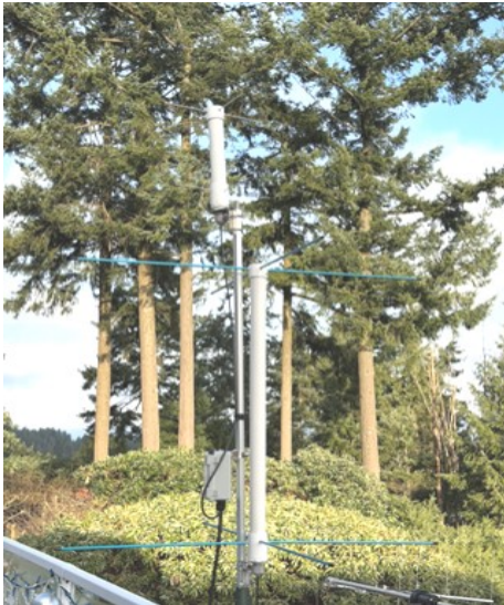
The UHF (top) and VHF (bottom) turnstile antennas in a temporary location on the deck at Bruce VE7PTN's QTH for testing.
