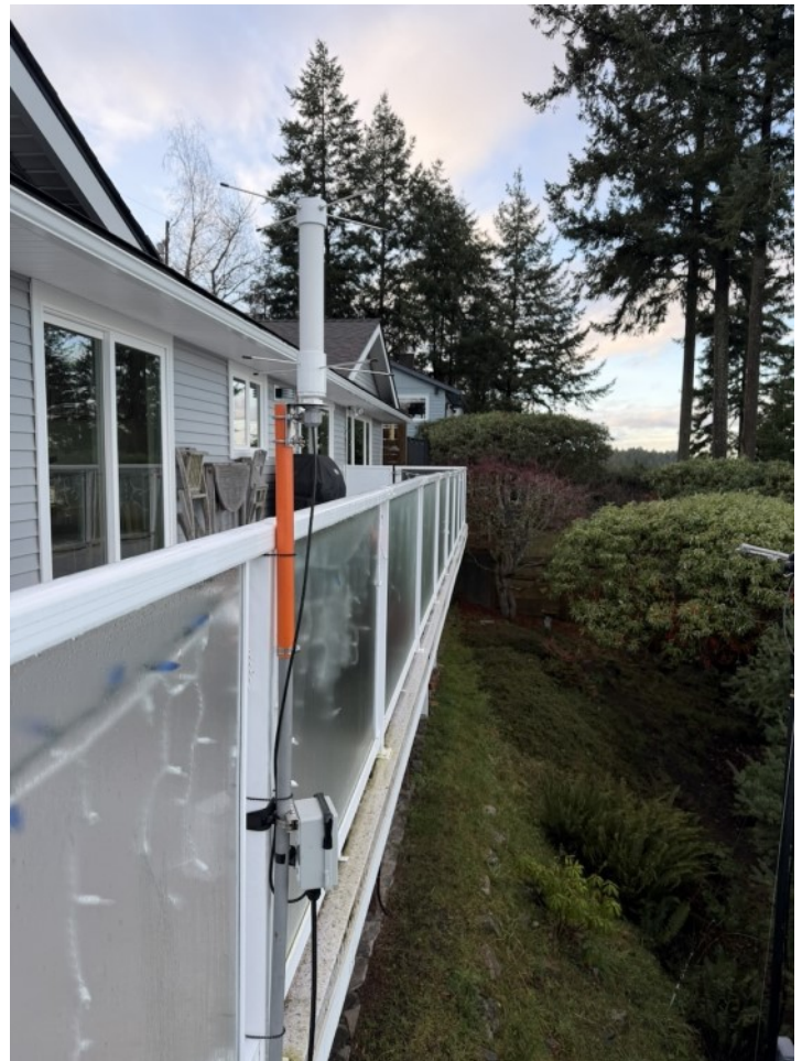
The UHF turnstile antenna and LNA in a temporary location on the deck at Bruce VE7PTN's QTH for testing. The roof gable in the background, just to the right of the antenna, is the planned location for permanent mounting.
