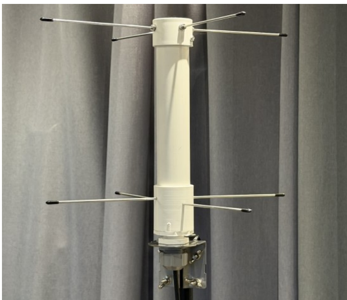
The UHF turnstile antenna built by Bruce VE7PTN using the design by Alicja Musiał posted at: https://alicja.space/blog/how-to-build-turnstile-antenna .
