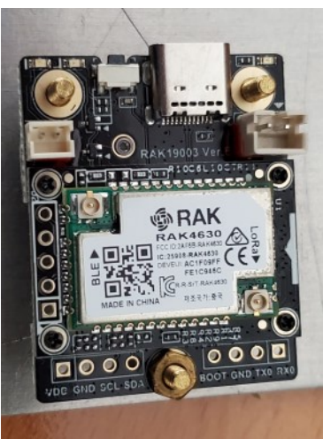
This is one of the low power devices which can be used as a node. This is the RAK 4630 module.
