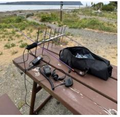
All-ICOM dual handheld radio satellite rig as tested during camping trip to Fillongley Park, consisting of IC-V86 for VHF uplink and ID-52 for UHF downlink and QSO recording. The storage bag for the rig is also visible; both radios, cables, and the collapsed antenna easily fit inside.
