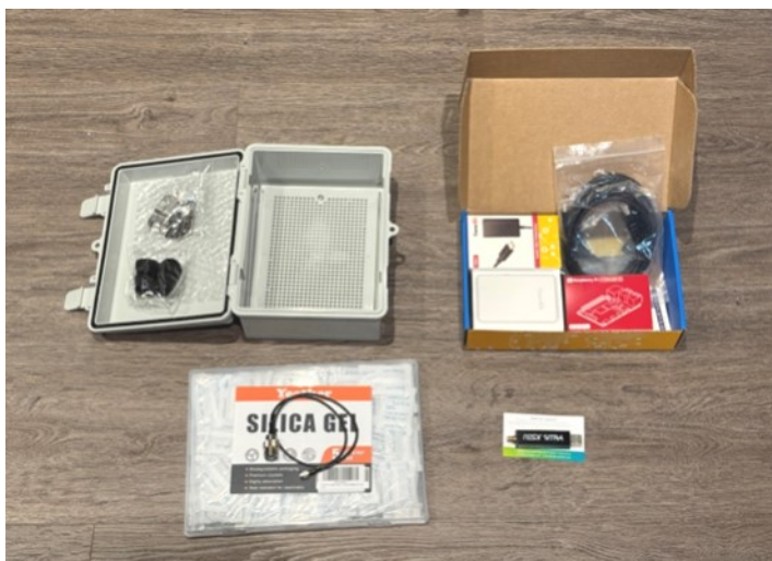
The components for the SatNOGS basic omnidirectional station being set up by Bruce VE7PTN. The computer is a Raspberry Pi 4 Model B in a kit from CanaKit ( https://www.canakit.com ) and the SDR is a Nooelec NESDR SMARt v5 SDR ( https://www.nooelec.com/store/sdr/sdr-receivers/nesdr/nesdr-smart-sdr.html ).
