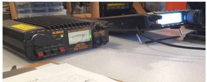
The VE7NA NVIS station ran a Yaesu FT891 at 100 watts to a dipole at 14m above ground.
