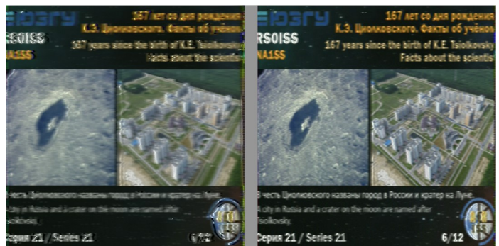
A comparison of SSTV decoded with noise reduction enabled (on left) and disabled (on right) on the receiver. The image without noise reduction applied to the FM signal results in a clearer SSTV decode.
