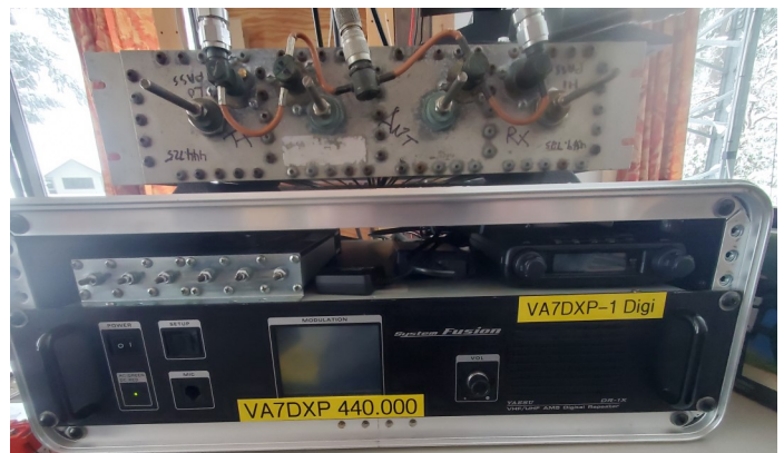
The VA7DXP portable Yaesu repeater was pressed into service to provide a temporary ITS link between Nanaimo and Victoria.
